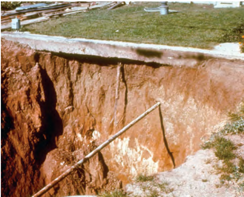
Ground failure caused by the collapse of a coal mine in Lafayette, Colorado.
